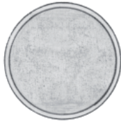
Erosion still permissible, plate can be polished
